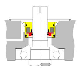
**ISOMAG** bearing seals eliminate the problems caused by leaking upper gearbox lip seals.
